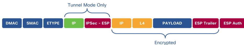
DIAGRAM IPsec frame format
