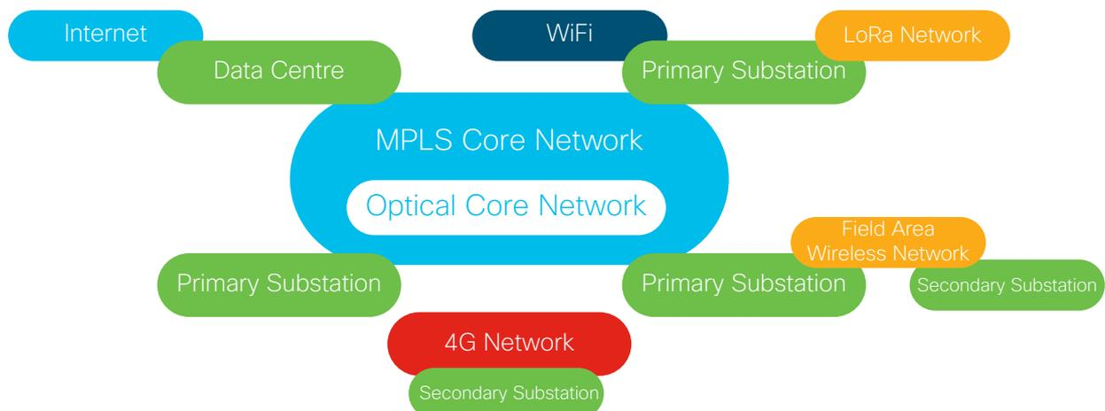
Figure 3 - High level architecture of the installed communication platform in PNDC
